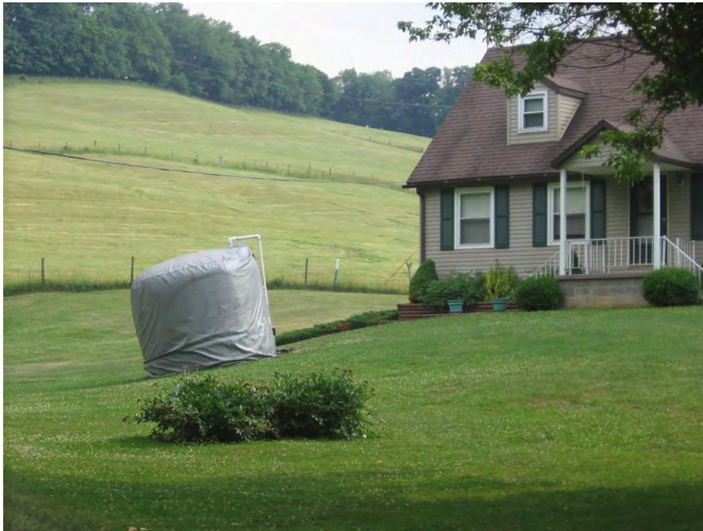
**FIGURE 17: A “water buffalo” in southwestern Pennsylvania. Plastic covered water tanks like this one often are provided by mining companies to serve as a temporary water supply after undermining has dried up the landowner’s well or spring.**
